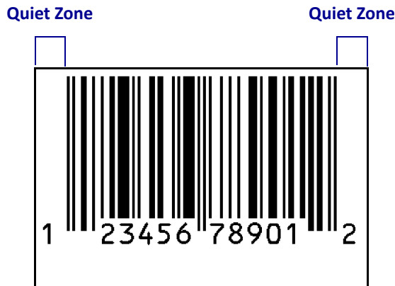
Figure 6 • Quiet Zone in a Bar Code
