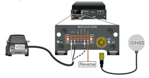
• **SharpX:** The GNSS connector is located on the ALPR Processing Unit face plate.
