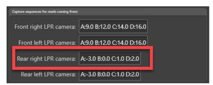
• Context camera A is triggered 3 meters before the plate read (-3.0).
