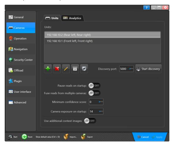
3 Make sure each camera in the **Units** list has the correct orientation. To do this, click on a camera, click the **Edit** button (), and then change the orientation of the camera to match where it is located on the vehicle.
