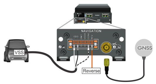
• **SharpX:** The GNSS connector is located on the ALPR Processing Unit face plate.
