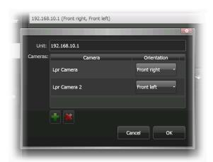
**NOTE:** Depending on the hardware installed, you might see up to two cameras (SharpZ3) or four cameras (SharpX) controlled by a single unit. For more information on camera options, see the *Deployment Guide* for your SharpX or SharpZ3 system.
