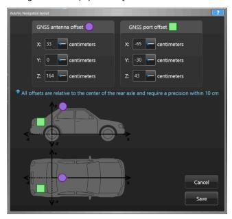
**GNSS antenna offset:** The purple dot on the graphic represents the position of the GNSS antenna installed on the patrol vehicle. Enter the following values (in centimeters) to configure the antenna layout:
