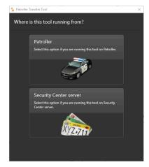
3 The tool guides you through the process of selecting your ALPR Manager root folder (in Security Center), selecting your USB media device, and starting the file transfer.
