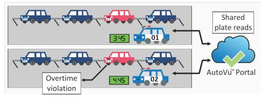
**NOTE:** If a long-term overtime rule is configured, you can use Plate link to connect multiple vehicles monitoring a single long-term overtime zone. For more information, see Configuring long-term overtime settings on page 69.
