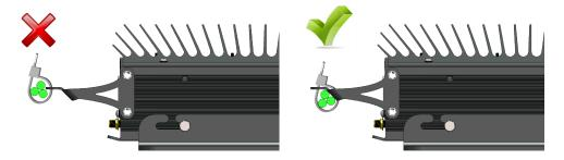
• For a cleaner installation, secure camera cables to the top of the cable rack and secure expansion module cables to the bottom of the cable rack.
