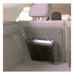
• Use appropriate screws to attach the bracket to the vehicle: ¼"-20 or M6. The screws must be long enough to secure the hardware, but short enough not to damage any vehicle components under the mounting location.
