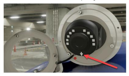
**TIP:** You can adjust three axes of rotation.
