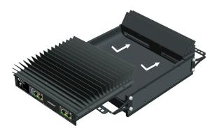
2 Firmly press the module to ensure that the connection at the back of the module is solid.
