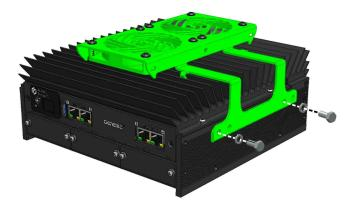
4 Connect the cooler pack cable to the **CP** plug on the back of the base unit.
